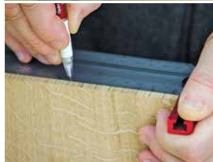
Using an INCRA T-rule for progressive markings
