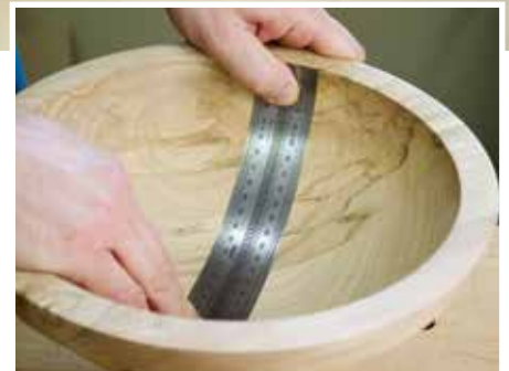
Using an INCRA flexible rule to measure inside a bowl
