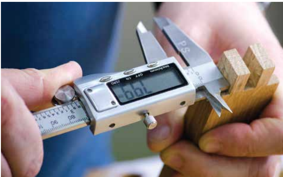
A GemRed digital Vernier calliper checking thickness
