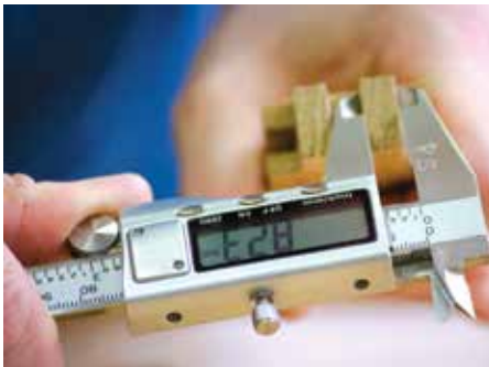
A GemRed digital Vernier calliper checking thickness
