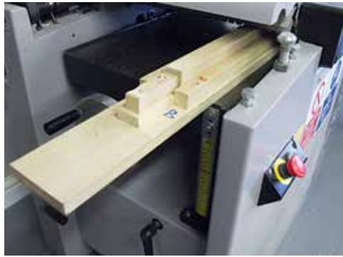
A taper jig on the thicknesser gives a clean finish but requires several passes to reach the finished size
