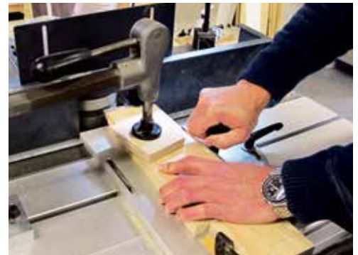
Tenoning on the spindle moulder gives clean and repeatable sloping shoulders
