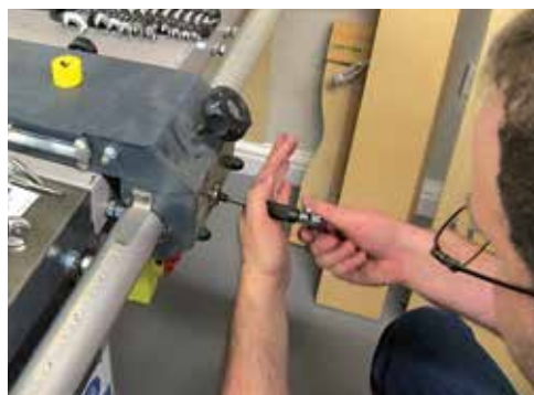
Re-tapping and cleaning the saw fence's threaded locking mechanism
