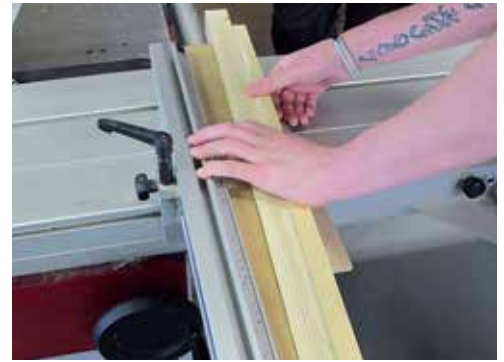
Cutting legs to length on the tablesaw with compound angles
