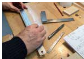
Measuring the tenon shoulders
