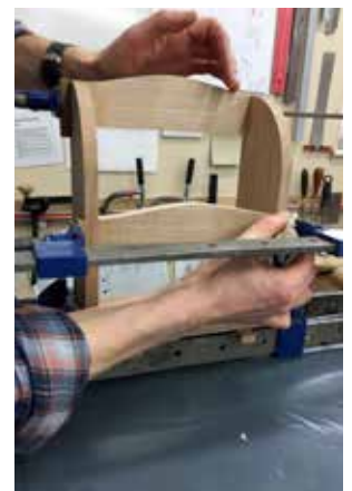
A damp cotton cloth removes excess glue from the tenons
