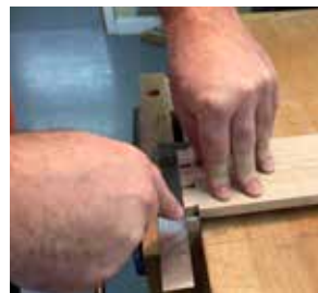
Scribing around the tails with a scalpel
