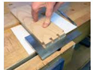
Paper shows the shoulder is tight to the timber while the square keeps it accurate
