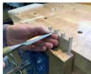
Chiselling down the shoulders between the pins
