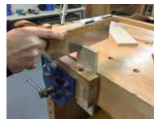
Brass-backed dovetail saw cutting on the waste side of the pins
