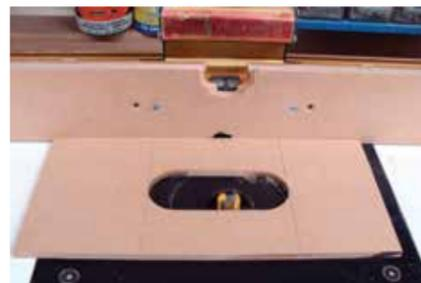
Moving the workpiece from right to left and progressively moving the fence further back until a smooth straight edge is formed
