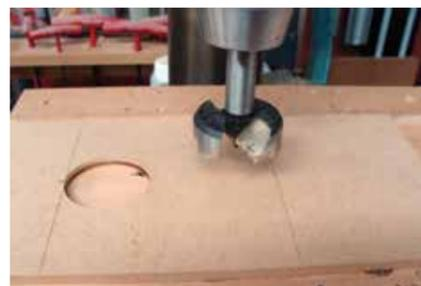
Using Forstner bits to cut the round ends of the handhold
