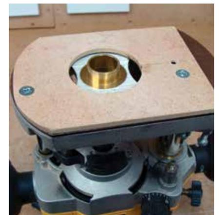
Fitting a false baseplate to overcome the excessive depth of the guidebush is simple
