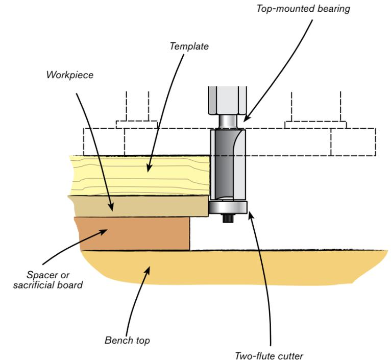
A typical setup for working with a template and bearing-guided cutters with a hand-held router on top of your workbench
