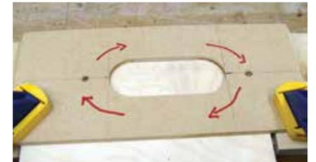
Master jig temporarily fixed to the blank production jig
