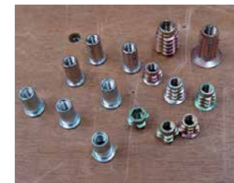
A mixture of threaded inserts with or without flanges and, on the left, rivet nuts; these are intended for insertion in sheet metal with a heavy-duty hand riveter, but which can also be used in wood. All the types shown have M6 threads
