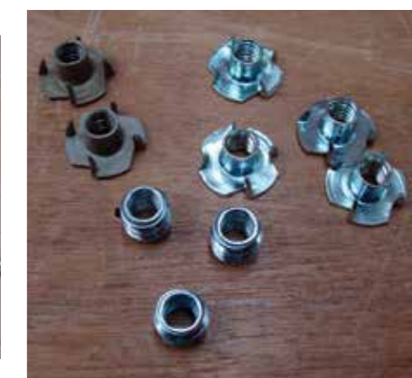
UNC versions of captive nuts for wood and plastic
