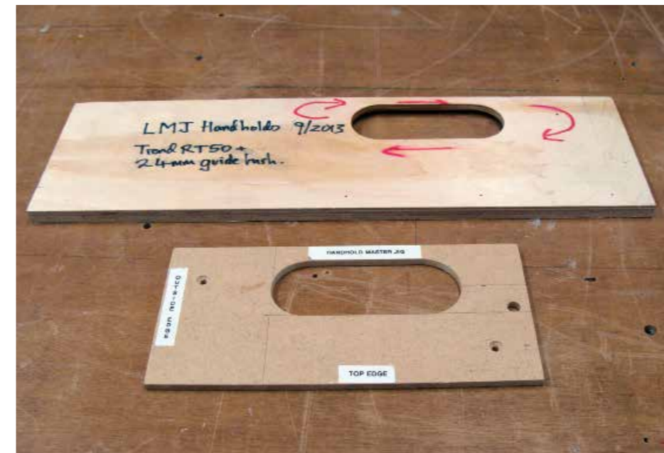
A master jig will benefit from as much information as possible relating to its orientation as well as its intended use
