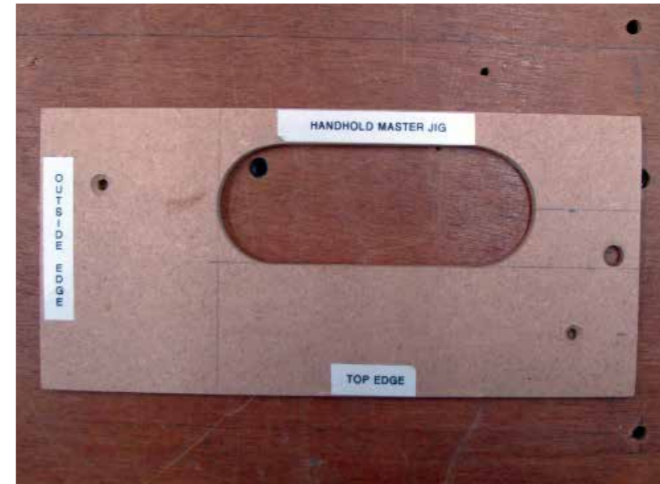
A master jig will benefit from as much information as possible relating to its orientation as well as its intended use
