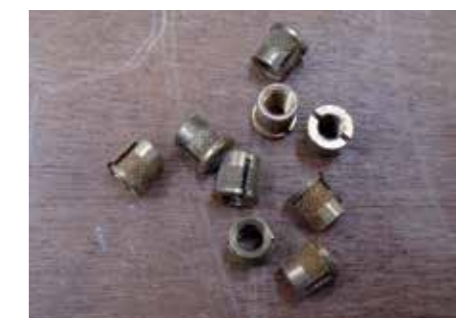
Another type of threaded fixing, this time for plastic and Tufnol
