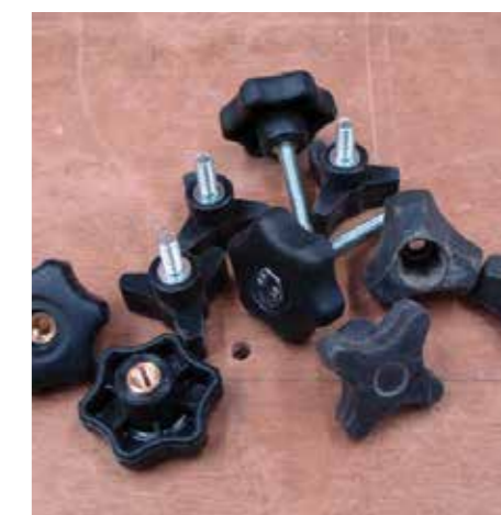
These handwheels are all M6 and are widely available, as well as being included in some jig hardware kits
