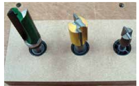
The cutter shown on the left does not have a plunge capability, but the two to the right can both plunge and cut on their sides
