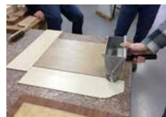
The gravity feed roller applying an even layer of UF adhesive
