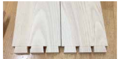
A pair of through dovetails with the cathedral grain rising from the joint
