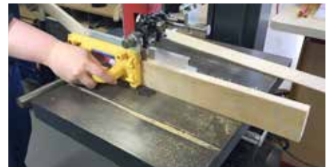
Deeping is often safer on the bandsaw, using a gripper to hold timber against the fence
