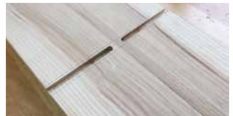
A pair of left- and right-hand rack sides with dovetail housings and matched grain
