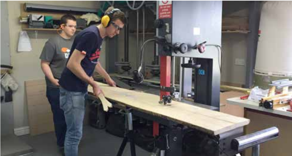
Freehand ripping a board in half following a chalk line
