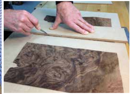
The veneer was cut and jointed together
