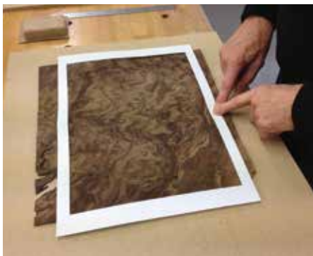
The window method was used to check how the veneer would look on the box
