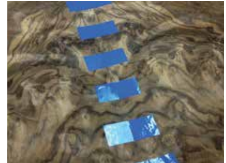
The joints were held with veneer tape
