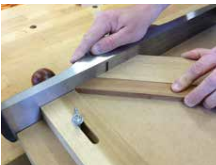
Using a WoodRiver No.7 plane on a 45° shooting board
