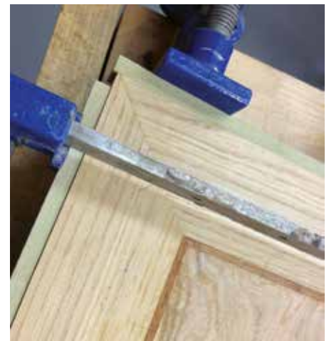
Using a pair of sash cramps to pull the mitres together
