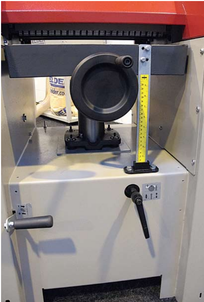
The thicknesser bed rises on a heavy single column and can be locked in position for accuracy
