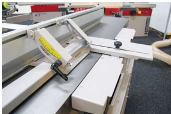
The newly designed fence adjustment and rear bridge guard
