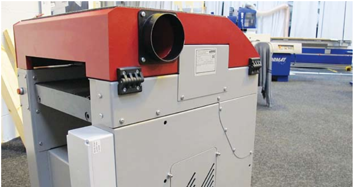
The 120mm dust extraction port is out of the way around the back of the machine
