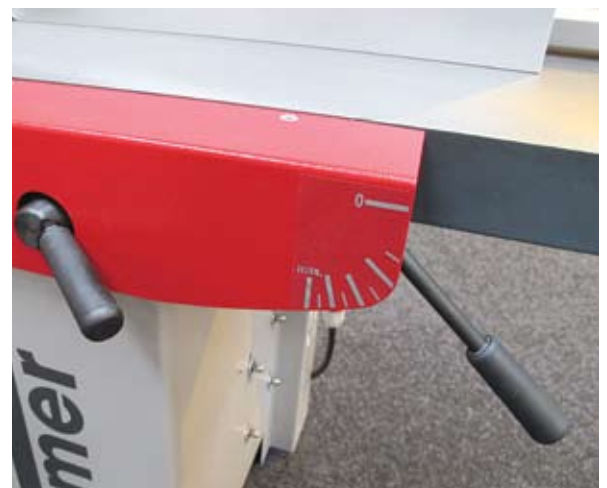
A lever easily adjusts the infeed table with a 0-4mm scale
