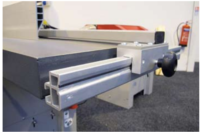
The fence is attached to an extruded aluminium bar on the end of the infeed table
