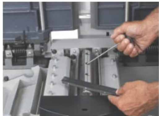
The three knife self-setting cutter block system
