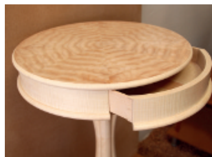
The cobweb veneer work and dovetailing give Simon Morrison's Shamshir table a classy finish
