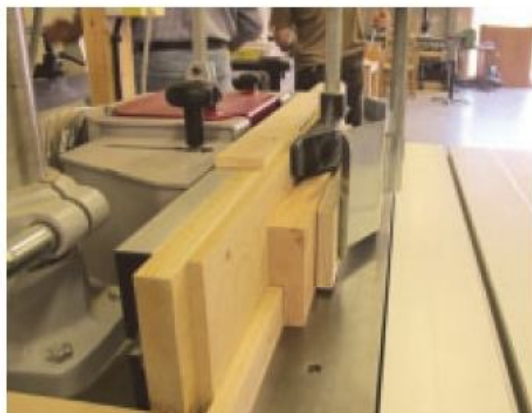
I have adapted my front Shaw guard with the addition of a piece of waxed plywood to give even pressure
