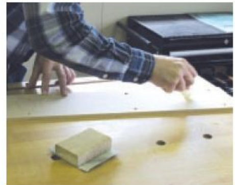
A swirl of wax is burnished to lubricate the false fence
