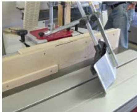
A saddle has been screwed to the false fence. Now we need to position the Shaw guards and break through the false fence
