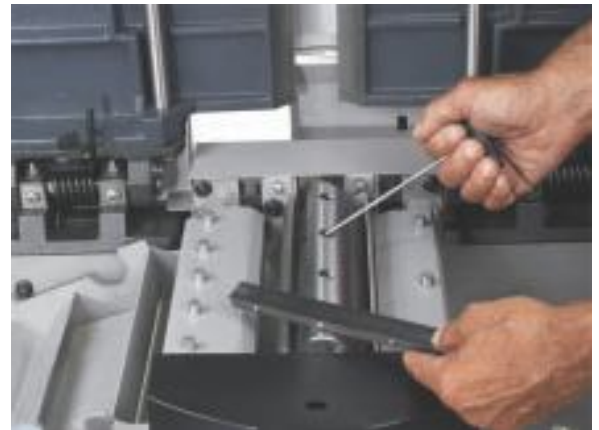
The three knife self-setting cutter block system
