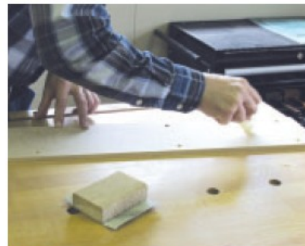
A swirl of wax is burnished to lubricate the false fence
