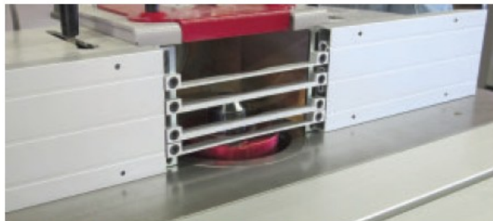
I use Hammer safety bars on my machine, which are quick and safe to set up plus there is no loss in the usable diameter of the tooling
