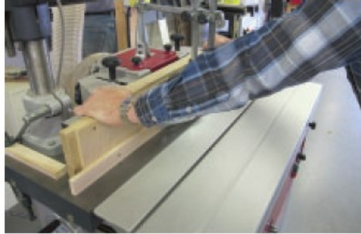
A pre-set pair of wooden blocks are behind the fence to act as a stop when the fence is in the correct position
