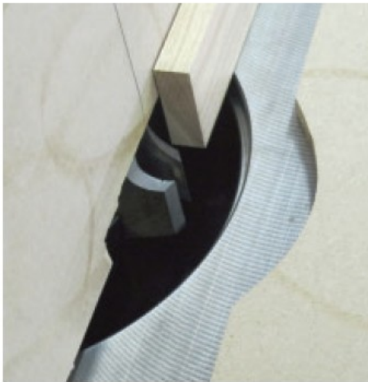
I use an MDF baseboard when the cutter block diameter does not suit standard table rings
