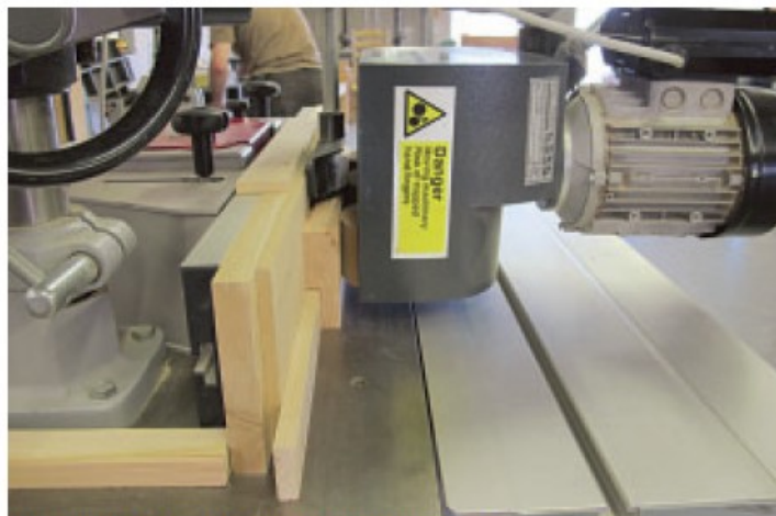
The power feed being used in conjunction with the Shaw guard
