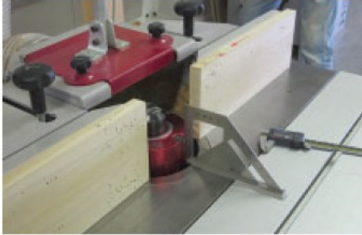
The height of the spindle block is set 1mm higher than its finished position, before attaching the false fence
